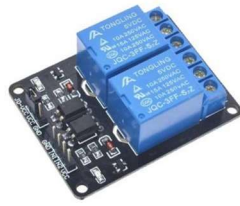
Gambar 2.15 Modul Relay 2-Channel
