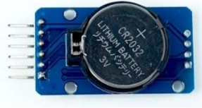
Gambar 2.16 Modul Real-Time Clock RTC DS3231
