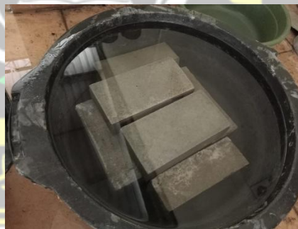
Gambar 3.18 Proses Perendaman Paving Block
