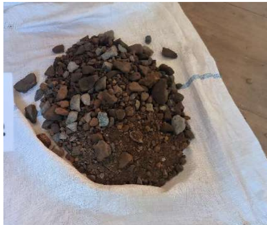
Gambar 2. Pencampuran Stone Crusher Waste + Tanah Asli
