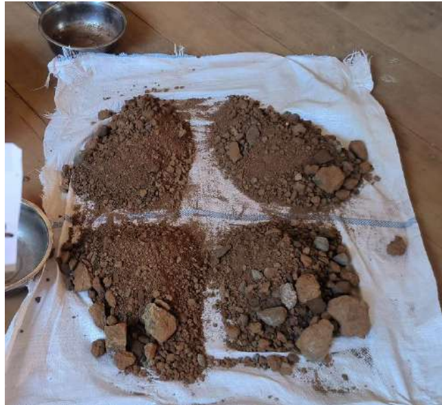
Gambar 3. Quartering Stone Crusher Waste + Tanah Asli
