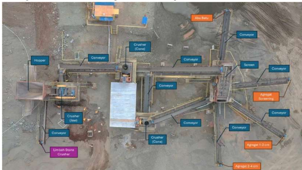
Gambar 2.2. Bagian-bagian Stone Crusher (IGP Bahodopi Block 2 & 3)
