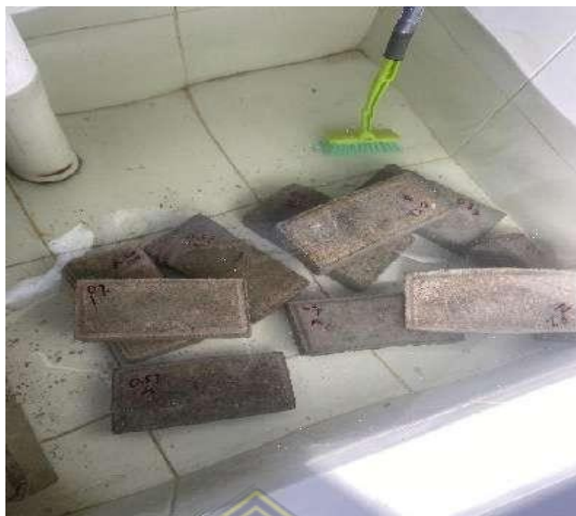
Gambar 4. 14 Perendaman paving block selama 24 jam
