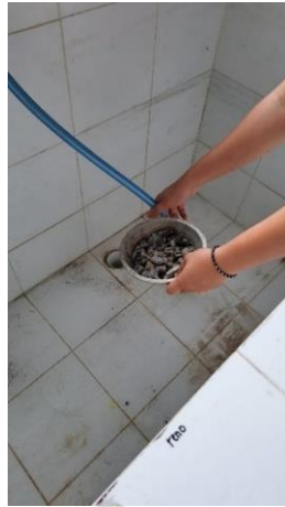
Gambar 4. 7 Kadar Lumpur Agregat Kasar Cara Pencucian
