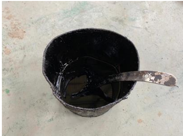
Gambar 4. 2 Aspal Penetrasi 60/70 Sumber : Hasil Penelitian, 2025
