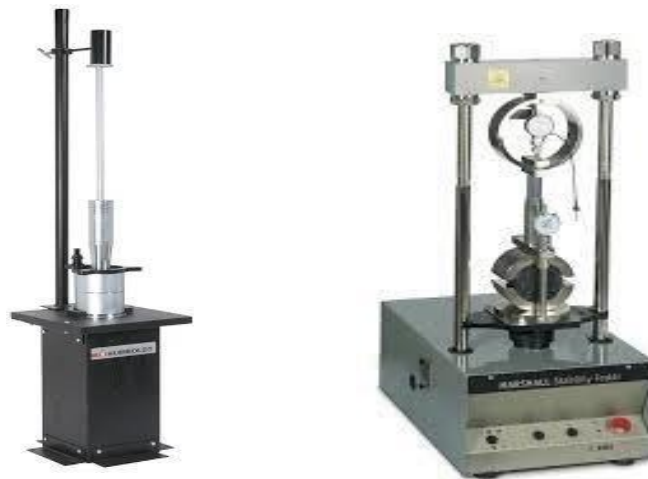
Gambar 2.1. Marshall Compaction Hammer dan Alat Marshall Test Uji Marshall
