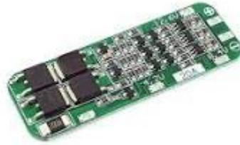
Gambar 2.13 *Battery Management System (BMS)*
