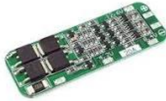
Gambar 2.13 Battery Management System (BMS)
