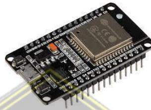
Gambar 2.1 Modul ESP32 Blink Kontrol
