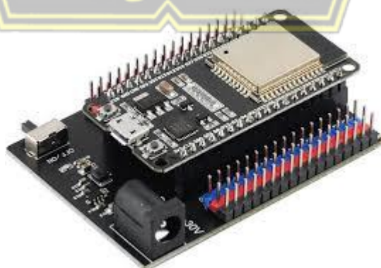
Gambar 2.2 Expansion Board ESP32 [13]
