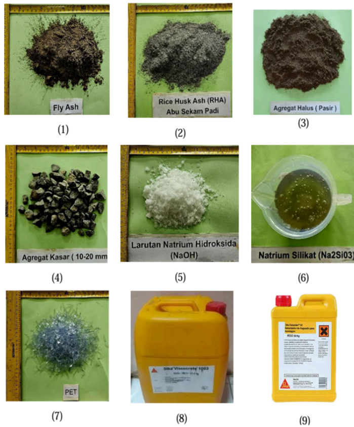
Gambar 3.1 Material beton geopolimer
