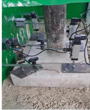
**Gambar 4.35:** Titik Monitoring *Settlement*
