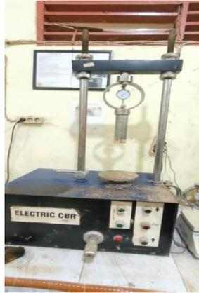
**Gambar 4.14:** Alat Uji CBR Laboratorium
