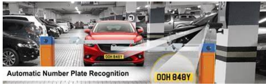
Gambar 2.3 ANPR atau Automatic Number Plate Recognition (Sumber: Google, 2024)
