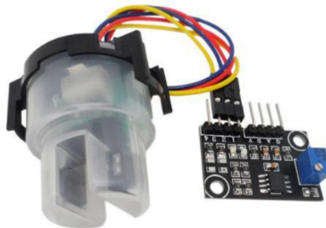
Gambar 2.8 Sensor kekeruhan (turbidity)
