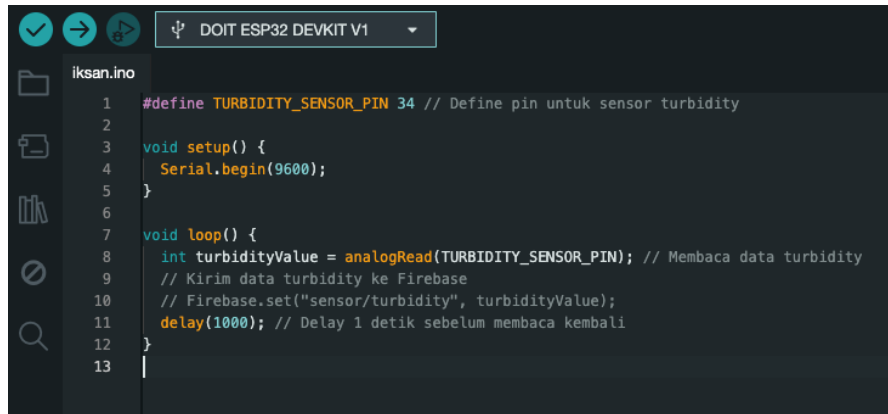
Gambar 3.6 Koding Kalibrasi Sensor Turbidity (Kekeruhan)
