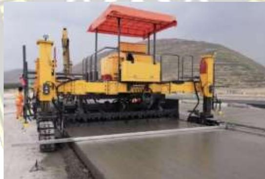
Gambar 2. 13 Concrete Slipform Paver
