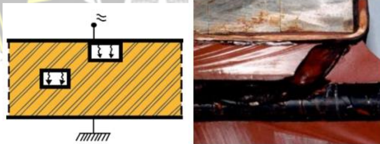
Gambar 2.6 Internal Partial Discharge [20]
