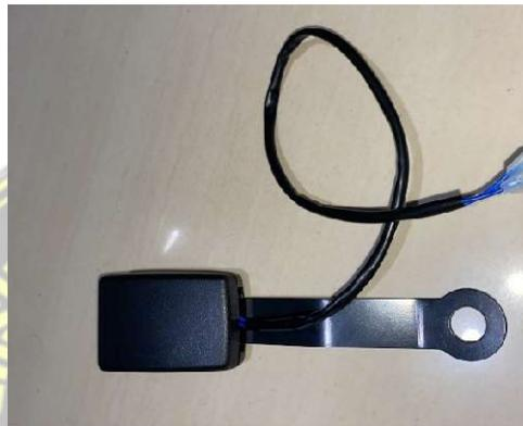
Gambar 2.6 *Sensor belt locking*
