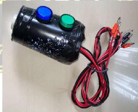
Gambar 4.3 Indikator pengingat alat *smart safety belt*
