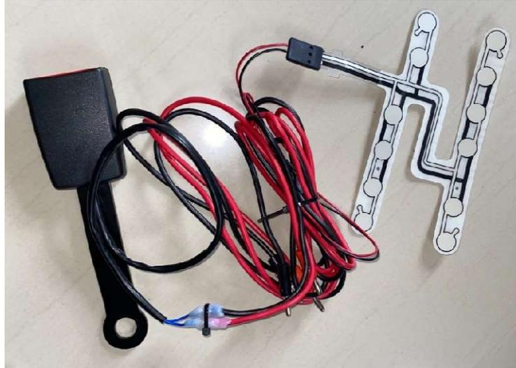
Gambar 4.4 Sensor *belt locking* dan sensor *membrane seat*
