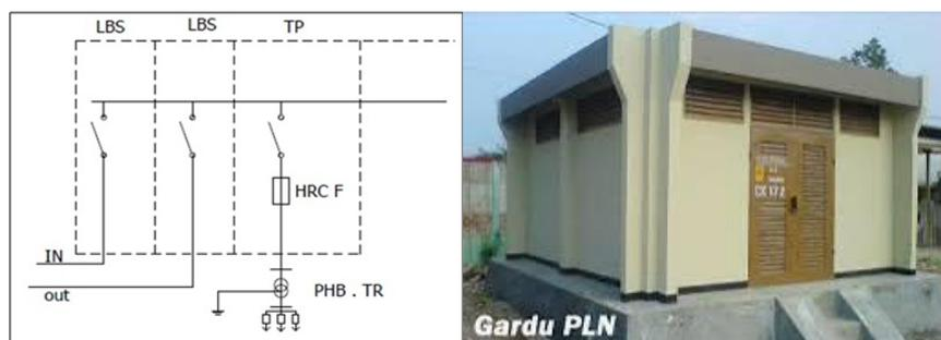
**Gambar 2. 4** Single Line Diagram Gardu Beton
