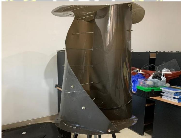
Gambar 3. 1 Turbin angin savonius heliks.
