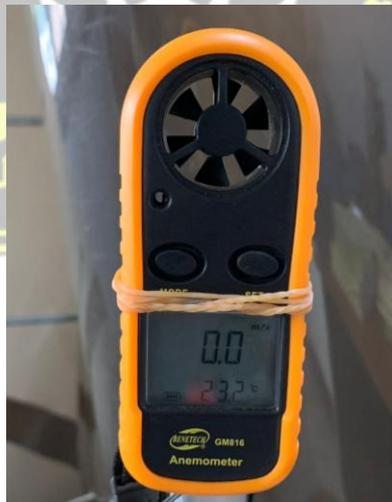
Gambar 3. 8 Anemometer digital Benetech GM816.
