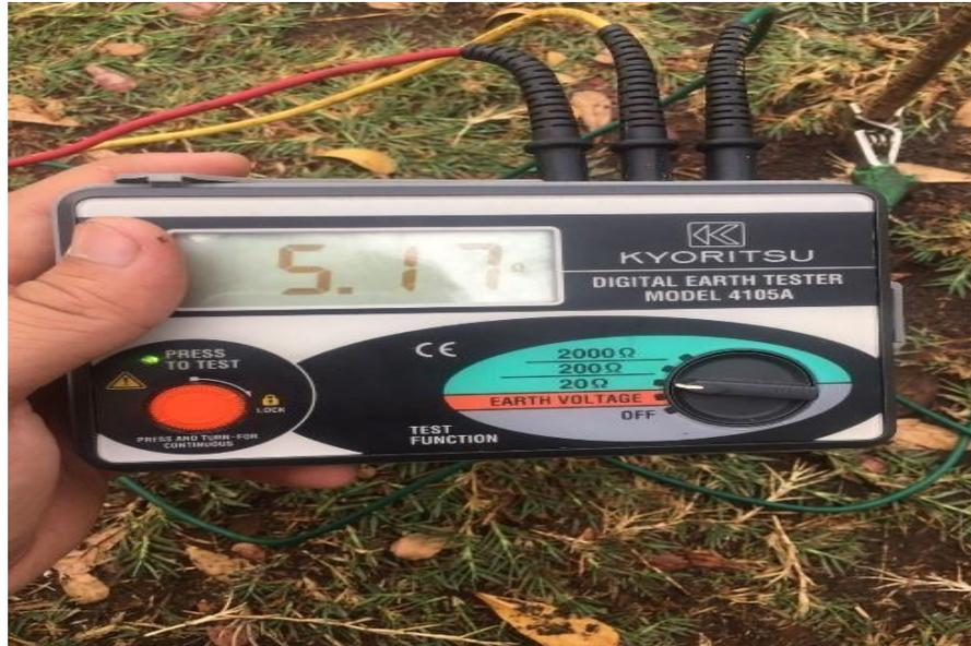
**Gambar 3. 5 Earth Tester Merk Kyoritsu-4105A.**
