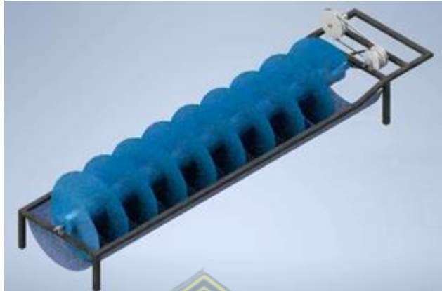
Gambar 4. 2 Desain 3D PLTMH tipe turbin archimedes screw.
