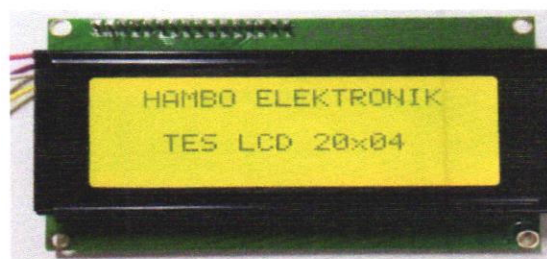
Gambar 2.5 Model LCD (Liquid Cristal Display).
