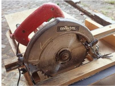
**Gambar 4. 8** Mesin *Circular Saw*
