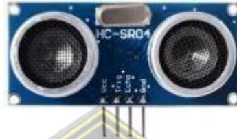
Gambar 2. 1 Sensor Ultrasonik
