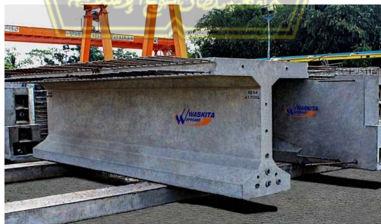
Gambar 2.4 Tampak T Girder
