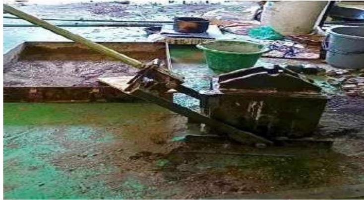
**Gambar 3.9.** Alat Cetak *Paving Block Press* Manual
