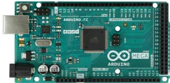
**Gambar 2.5** Arduino Mega 2560 [11]
