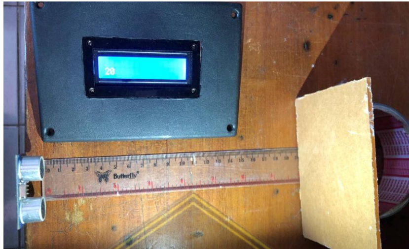
Gambar 4.16 Pengujian Sensor Ultrasonik HC-SRF04
