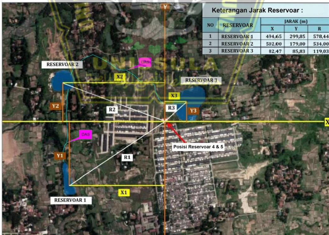
Gambar 4.21 Posisi Reservoir 1, Reservoir 2 dan Reservoir 3
