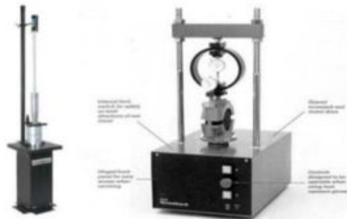
Gambar 2. 2. Marshall Compaction Hammer & Alat Marshall Test
