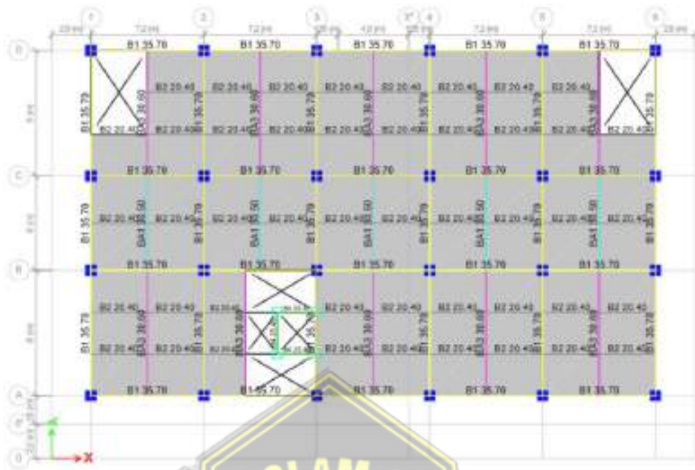
Gambar 4.45. Denah Balok Lantai 8
