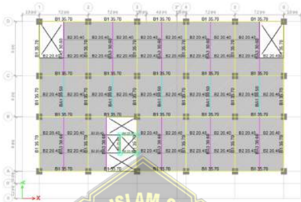
Gambar 4.41. Denah Balok Lantai 4
