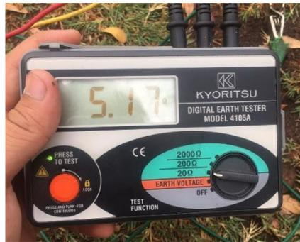
**Gambar 3.9** Earth Tester Merk Kyoritsu-4105A
