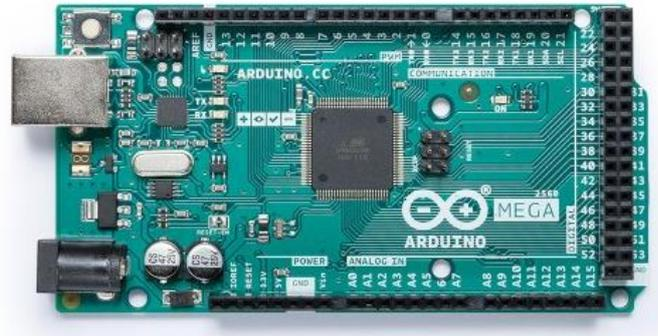
**Gambar 2.9** Arduino Mega [27]
