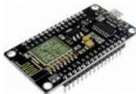
**Gambar 2.4** Modul NodeMCU Devkit V 1.0 [24]
