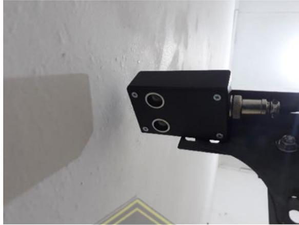
Gambar 4. 3 Sensor Ultrasonik
