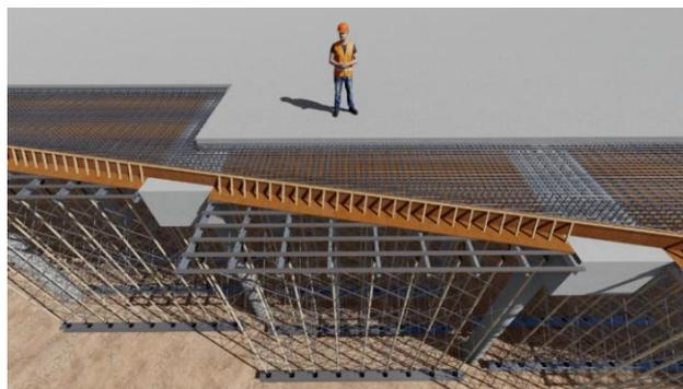
**Gambar 4.46.** Pembesian *Deck Slab*
