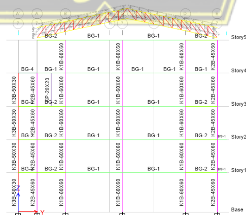
Gambar 3.23. Permodelan ETABS V.18.1.1 As 7 Gedung Bea Cukai Tanjung Emas
