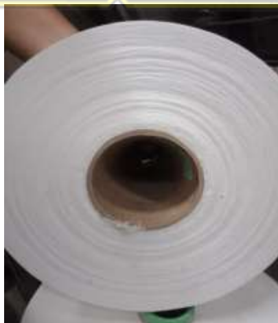
Gambar 4.14 Jenis Cacat Pattern Winding
