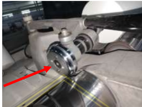
Gambar 4.31 Letak Cradle Bearing Center
