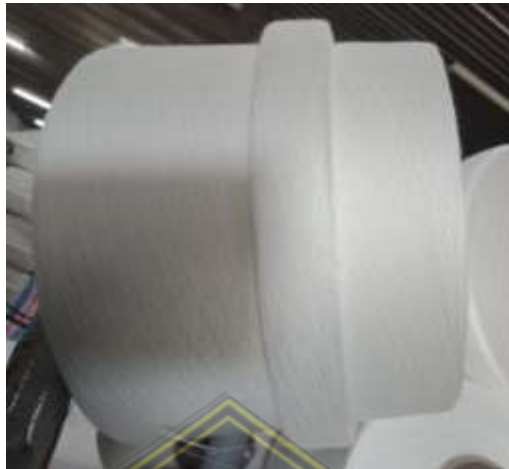
Gambar 4.12 Jenis Cacat Swelled Package
