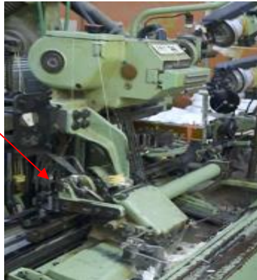
Gambar 4.8 Part Selector Weav
