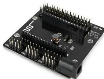
Gambar 2.7 NodeMCU Baseboard [18]
