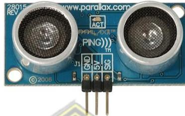
**Gambar 2.4** sensor ultrasonic PING [15]
