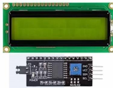
**Gambar 2.11** Liquid Cristal Display (LCD) 16 x 2 dan perangkat Inter Integrated Circuit (I2C) [28]
