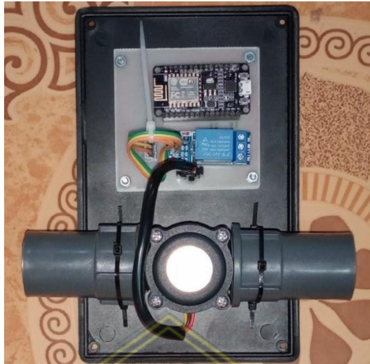
Gambar 3.5. Perancangan Water Flow Sensor.
