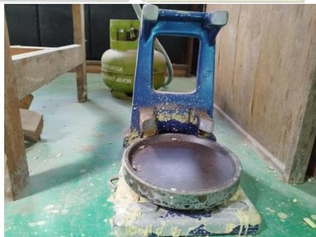
**Gambar 3.15** *Vertical Cylinder Capping*
