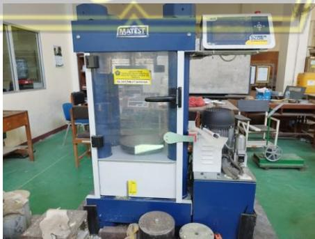
**Gambar 3.6** *Compressing Test Machine*
