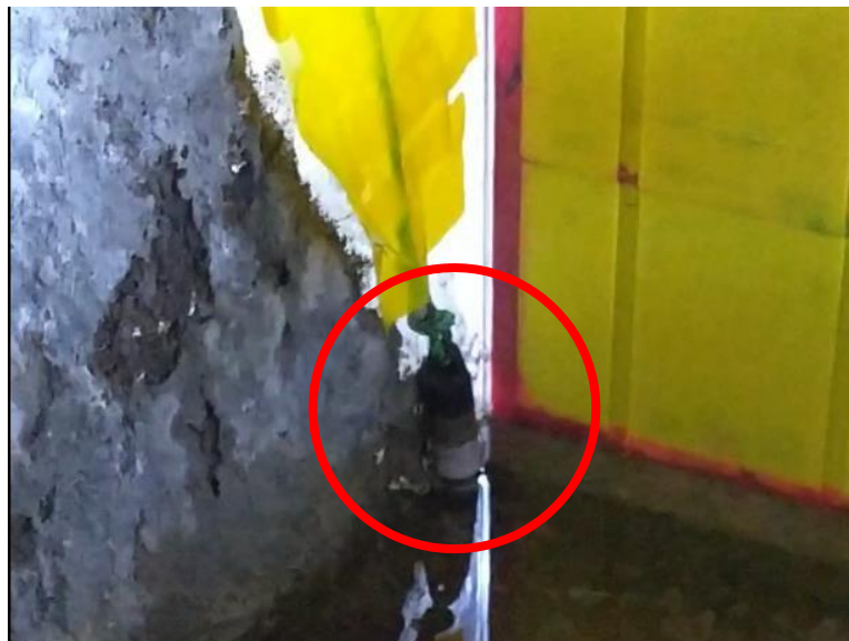
Gambar 3.8: Sensor Water Level
