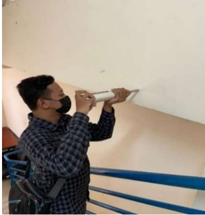
Gambar 4.4 Pengujian rebound hammer
