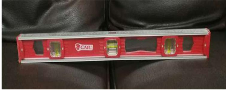
**Gambar 3.9** Alat waterpass manual
