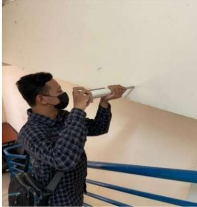
**Gambar 4.4** Pengujian *rebound hammer*
