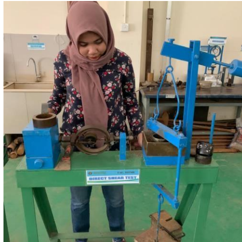
Gambar 3.10 Direct Shear Test
