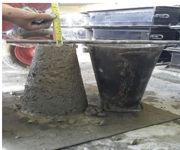
Gambar 4. 9. Hasil Trial Uji Slump
