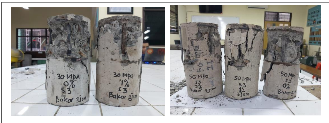
Gambar 5. 78 Keruntuhan Beton Serat Terkekang Bakar Senggang S100
