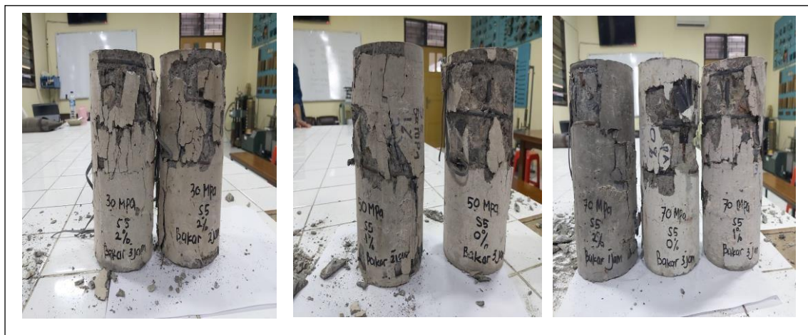
Gambar 5. 80 Keruntuhan Beton Serat Terkekang Bakar Senggang S50
