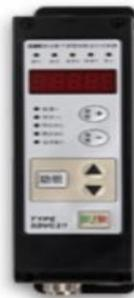
Gambar 2. 13 *variable frekuensi* digital controller [18]
