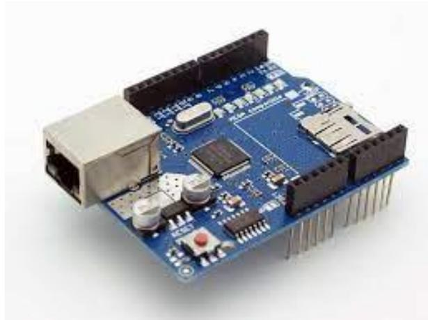
Gambar 2.11 *Ethernet shield* (Sumber : [www.store.arduino.cc](http://www.store.arduino.cc))
